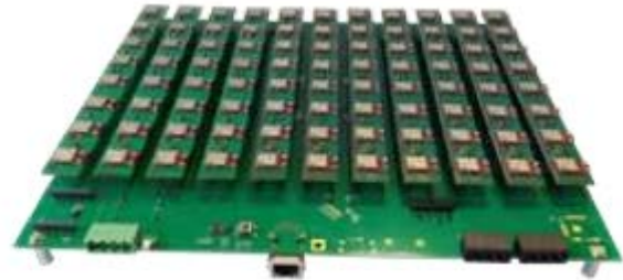
Figure 1 Fast spectrum measurement system (FSMS)
