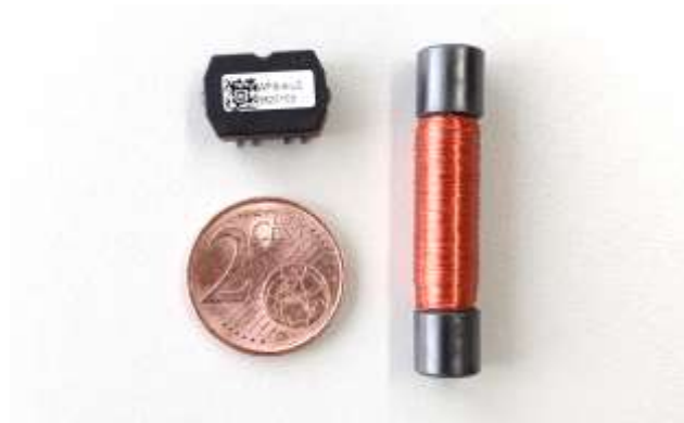
Figure 2 Wiegand sensor for energy-self-sufficient motion sensing (top) and Wiegand generator (right)
