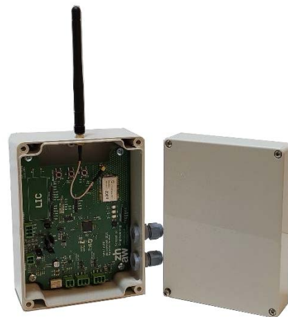
Figure 11 Prototype for monitoring infrastructure in urban water management includes energy harvesting, data acquisition, data analysis and data transfer in a waterproof housing. A solar cell was mounted to the cover.
