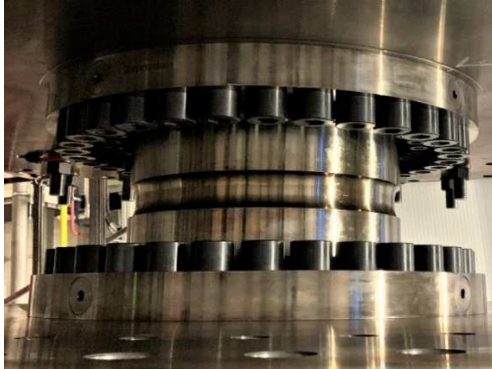
Figure 2 TTS installed in NTB between two adapters
