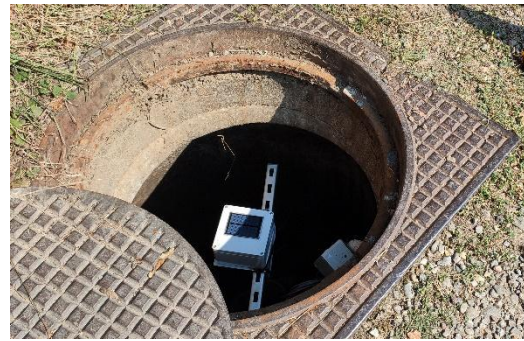
Figure 8 Prototype mounted directly below the ventilation hole of a manhole cover
