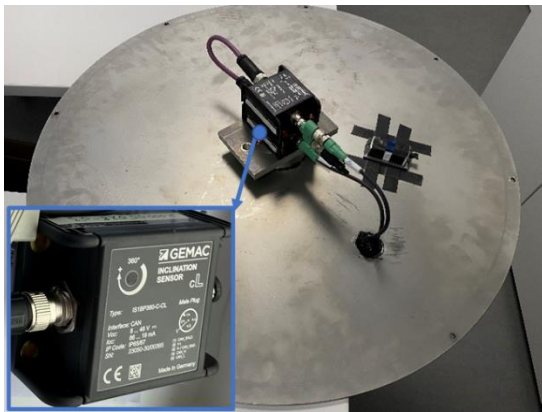
Figure 2 The inclinometer stack centred on the inner side of the TTS cover plate
