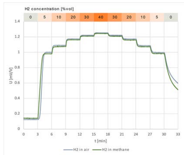
Figure 5 Supply voltage: 5V, flow: 80 sccm: increase in hydrogen concentration in air and methane from 0 to 40% vol% hydrogen
