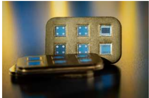
Figure 3: Hermetically encapsulated modules
