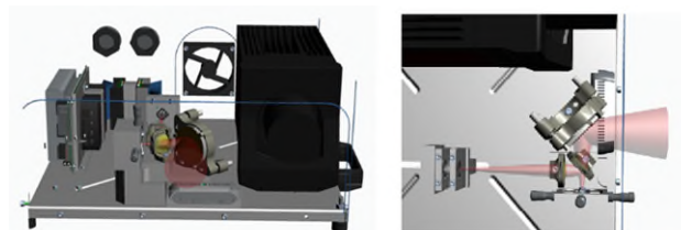
Figure 1 Left: Setup of the real time active gas camera. Right: Top view of the sketched laser light pattern in red. Less than 1% of the laser light is coupled out for locking the target gas line.
