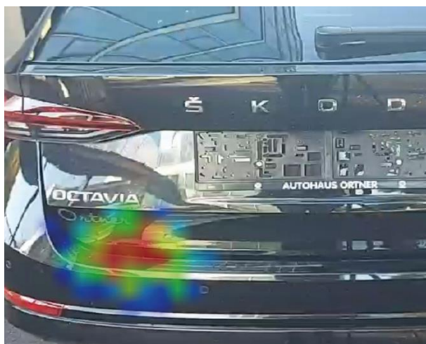
Figure 11. Leakage at the interface between the tailgate and the sill at 53,5dB with a dynamic range of 6dB.
