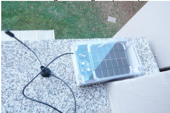
Abb. 5: Autarkes mobiles Multisensorbox
