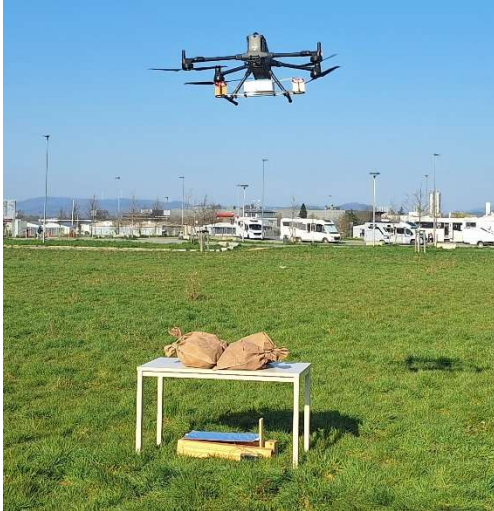
Fig. 6: Field tests with a DJI Matrice 400 drone, using the mechanically moving aluminium-coated plate as a breathing dummy. Here, bags with ceramic tiles are used as obstructions.
