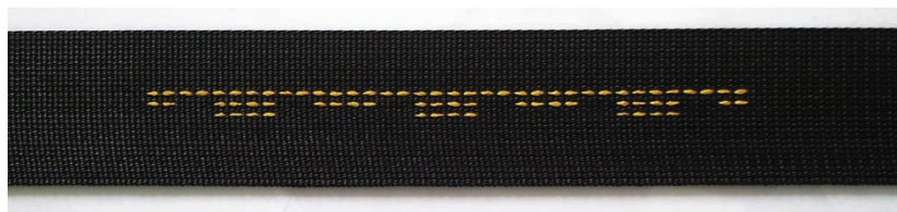
Figure 1: Safety belt with control tear strips for visual evaluation
