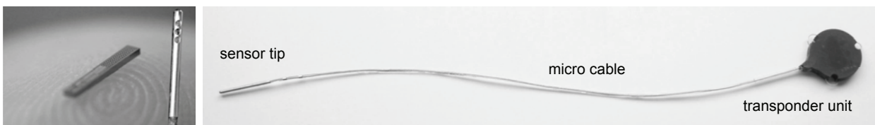
Fig. 9 Blood pressure sensor implant. Micrograph of the sensor tip and the tiny sensor chip (left), implant consists of sensor tip, micro cable and transponder unit (right).
