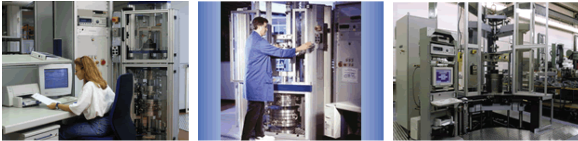
Fig. 5 Different force calibration machines for capacities 2,5kN; 25kN and 240 kN at HBM
