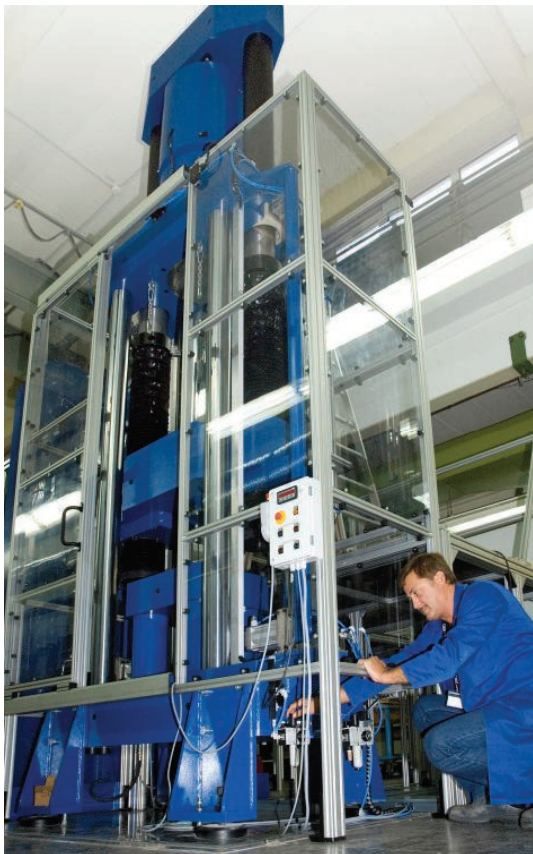
Fig. 6 Calibration machine with capability 5MN
