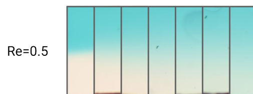
Fig. 5. Images of the channel contents for an ink dilution along a microfluidic Dean mixer at Reynolds numbers of 0.5. The channel positions match those in Fig. 2.
