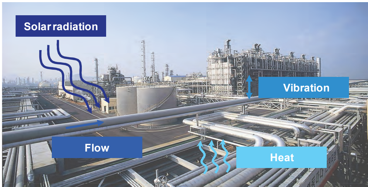
Figure 1: Energy harvesting converts ambient energy or energy available in the process itself into usable electrical energy.
