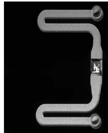
Figure 3: Picture of backside of the final flow sensor chip with meander fluid channel.
