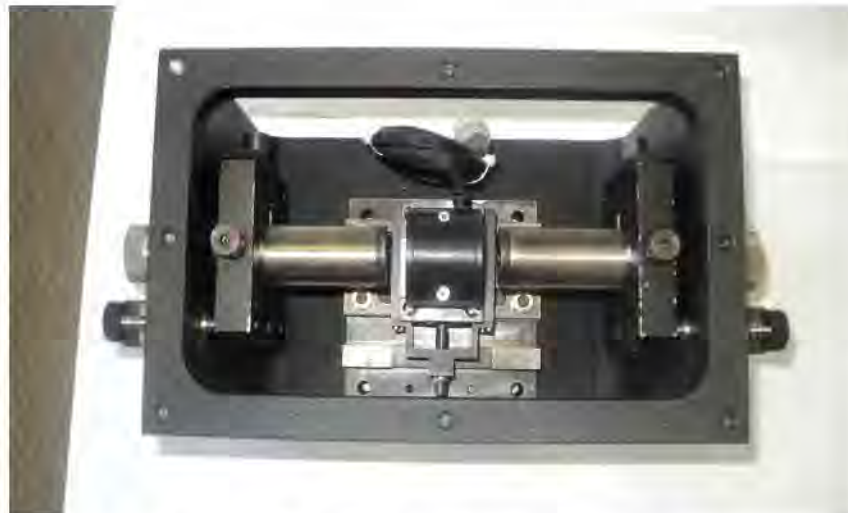
Figure 5 – The OPO monolithic cavity
