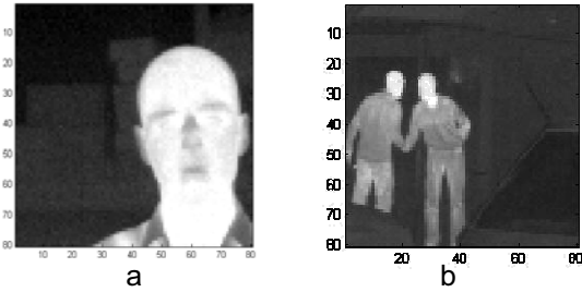
Fig. 7. Thermal imaging scene recorded using an infrared camera with 25 mm f/1 optic: 7a: distance 1m; 7b: distance 10m
