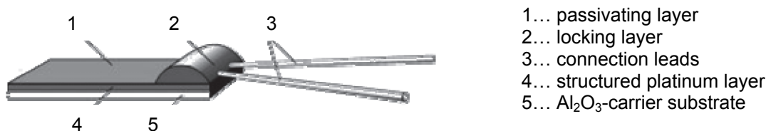
Figure 1: Structural design of a ceramic Thinfilm-Temperature sensor element
