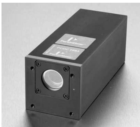
Fig.8: PCDC Module including CPM, high voltage power supply and readout electronics with USB interface
