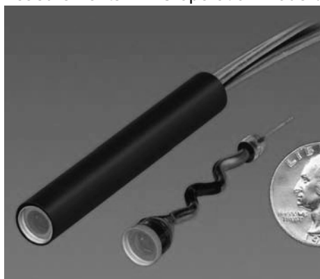
Fig.1: Photograph of the Channel Photomultiplier. Left shows the encapsulated CPM; at the right the bare CPM without encapsulation is shown.
