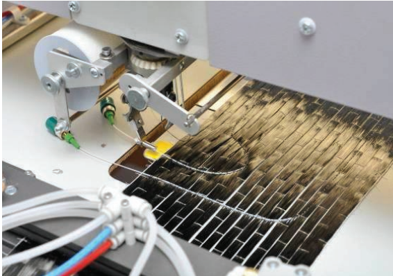
Figure 3: Embroidery of optical fiber on technical textile (carbon fiber clutch).
