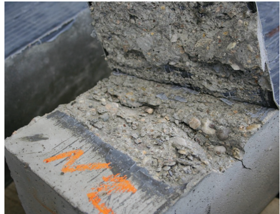
Figure 1: Destroyed concrete beam after failure of CFRP material.
