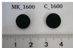
Fig. 2 Samples of the C/SiOC pellets with d = 10 mm diameter.
