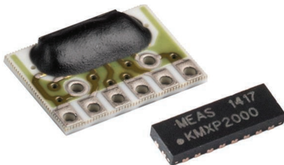
Figure 6 Comparison between COB based chip assembly on ceramic and DFN package
