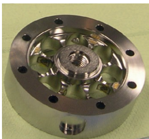
Fig.1: A spring body of a radially symmetric shear-force transducer. The strain gauges are glued on the bars in a way that there is always one strain gauge picking up the negative strain and another one picking up the positive strain. The Wheatstone bridge circuit compensates the temperature influence on every single bar so that the sensor has an excellent behavior under temperature gradients.
