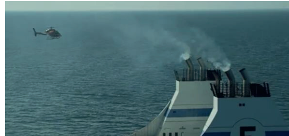
Fig. 4. Field testing includes monitoring of ship fumes aboard the coastline of Denmark by the Explicit company (May 2020).
