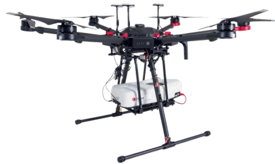
Figure 3: Commercial drone equipped with the methane spectrometer.
