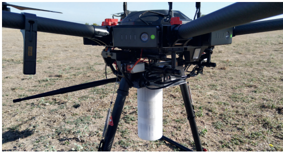
Fig. 1. The radiation monitoring system mounted onto a DJI M600P drone.
