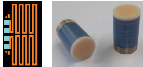
Fig. 5. Realized adjustable high temperature reference areas. Left: screen-printed layout of orange heater area and blue interconnection pads, right: realized functional samples with blue insulating surface coating.
