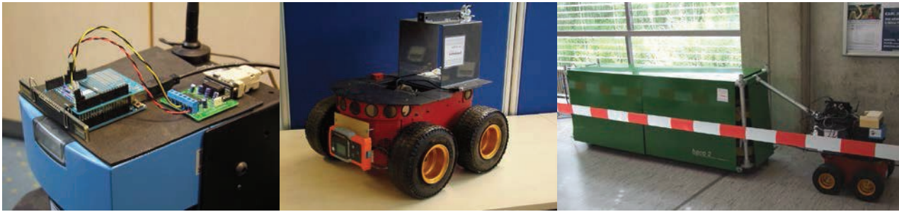
Figure 9: a) Prototype of the low cost laser sensor, b) Robot with attached commercial laser receiver, c) Prototype of the line coating robot
