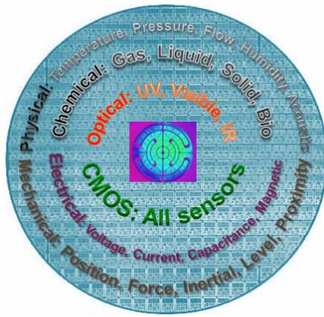
Fig 1: Types of sensors that fabricated on CMOS silicon wafer
