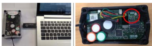
Fig 9: Combined EC and MOX sensor module
