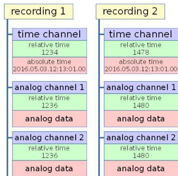
Fig. 2 Packet structure of two IRIG106 CHAPTER 10 recordings.
