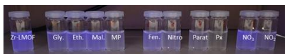
Fig. 3. Photoluminescence responses of Zr-MOF against 10 organophosphates compounds containing nitro group. The final concentration of all the compounds is 0.012 mM.
