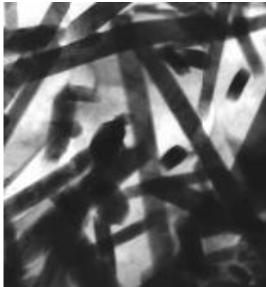
Fig.2. Crashed SbSI crystals used for thin film thermal deposition.
