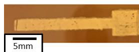
Fig. 3. Deposit of 60 layers of particle free gold ink after thermal treatment at 350°C for 2 hours
