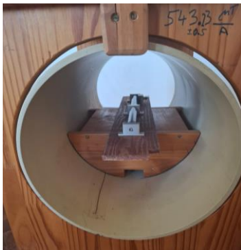
Fig. 2. Torque rod inserted in solenoid centre
