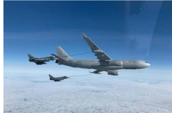
Fig. 2. A330-MRTT aircraft refuelling two fighters through the underwing pods
