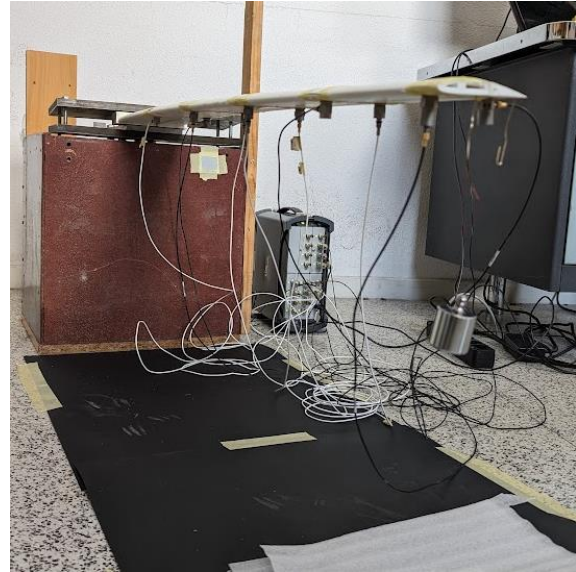
Fig. 12. Accelerometers in the lower surface to measure the dynamic tests response
