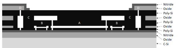
Fig. 2. Schematic cross section of the sensing structure with stiffening structure and sense capacitance (A), reference capacitance (B) and membrane suspension (C).
