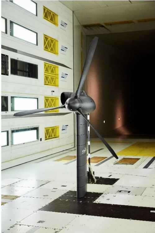
Figure 1: The ATTILA model in the LLF at DNW Marknesse, Netherlands
