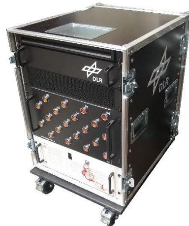
Figure 9. TEDAS 3 rack system.
