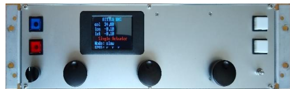
Figure 11. ATTILA HMI system – pitch control.
