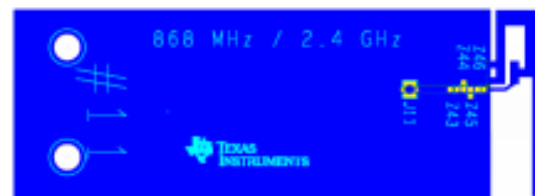
Figure 5. 2.4 GHz antenna test board
