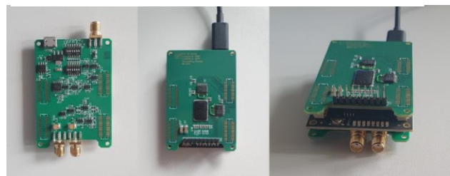
Figure 2 Eddy current transceiver, ASIC-PCB and completely stacked sensor-system
