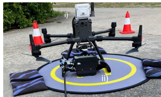
Figure 1. DJI Matrice M300 RTK with i) Sniffer4D ii) SJH-5 and SCD30 sensors.
