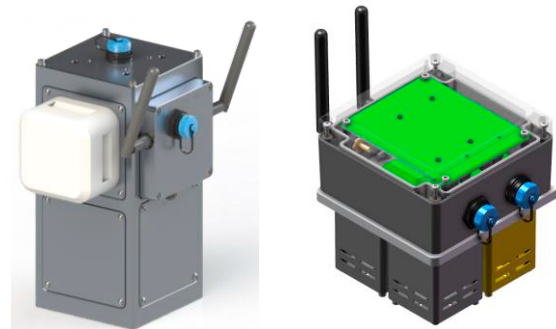
Fig. 3: Different concepts for a modular sensing node. The left picture shows a system where two different modules are attached to the core 'tower unit'. On the right, four sensor modules are attached underneath a main module.
