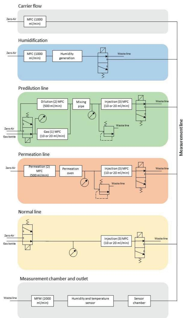
Figure 2 Overall schematic of the GMA based on [7]
