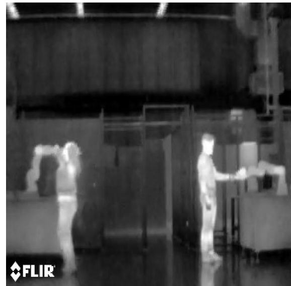
Figure 2: Infrared image in industrial settings with two cobots, moving human (left) and human cobot interacting (right).
