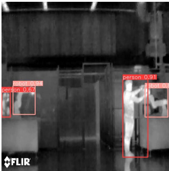
Figure 3: Results of the prediction with the YOLOv5n model, detecting occluded person and interacting person and both robots in different poses.
