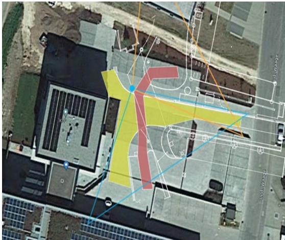
Fig. 1: Smart city campus test site plan of ZDE in Westhausen. The red area represents a cycle-foot path and the yellow area represents a street / Underground parking garage entrance. The blue- and orange line triangles indicate the visible areas of the observing cameras. (This figure was created by ZDE and contains material from Google.)
