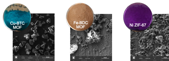
Fig. 1: appearance and SEM figure of MOF films.
