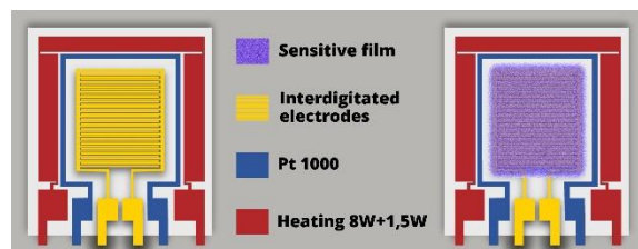
Fig. 3. Schematic illustration of the ethanol sensor.
