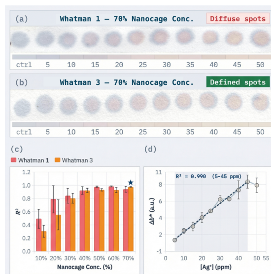
Fig 2. Optimization of paper substrate and nanocage ink for \text{Ag}^+ detection. (a) Whatman 1 at 70% shows diffuse spots from lateral wicking. (b) Whatman 3 at 70% shows uniform, well-defined spots. (c) R^2 of \Delta b^* vs. [\text{Ag}^+] for 10–70% nanocage concentrations on both substrates, with Whatman 3 at 70% selected as optimal. (d) Dose-response curve for Whatman 3 at 70% loading with linearity from 5–45 ppm ( R^2 = 0.990 ).
