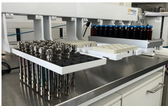
Fig. 1. Automated headspace sampling of volatile organic compounds produced by liquid bacterial cultures onto thermal desorption tubes.
