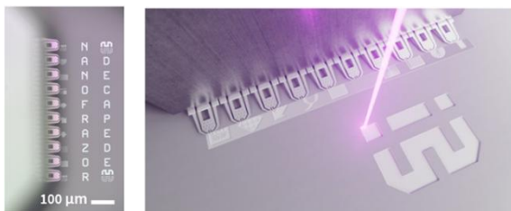
Fig. 1. (left) NanoFrazor in-situ microscope showing the Decapede over a resist-coated substrate, writing features in both 2D high-resolution and in grayscale. (right) Simulated image of the Decapede patterning different features, alongside the integrated laser writehead.
