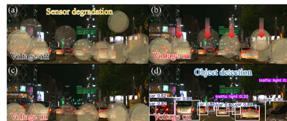
Fig. 3. Sequential snapshots of conductive and non-conductive droplet cleaning on L-DEP-based self-cleaning glass for autonomous driving optical sensors
