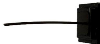
Fig. 1 Cilium ( d = 1 mm, l = 35 mm) fabricated in a mould-based approach.
