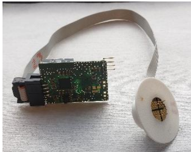
Fig. 2. Assembled patch connected to the mother board
