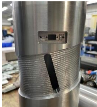
Figure 6: Front of machined surrogate body
