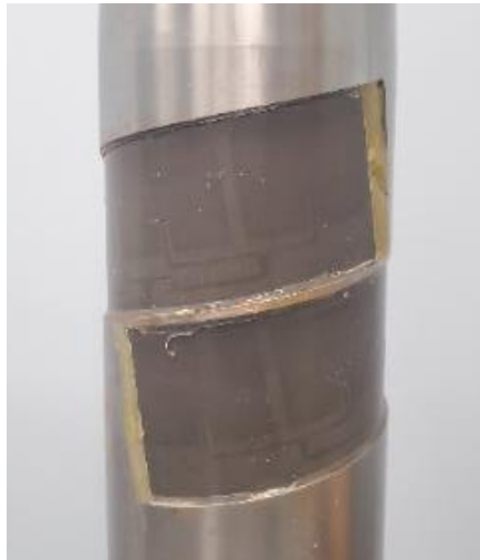
Figure 7: Rear of surrogate projectile with installed wrap antenna
