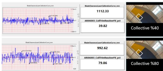
Fig. 13. Blade Clearance Behavior According to Collective Input
