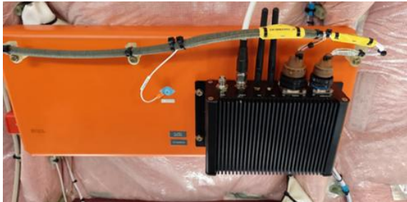
Fig. 6: PLANET 9770 FTI Equipment in A321neo
