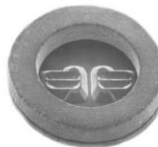
Photograph of diaphragm, glass-bonded to heavy silicon ring, 0.1 in (2.5 mm) O.D. by 0.02 in (0.5 mm) thick.
