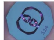
Photograph of diaphragm taken with scanning electron microscope 0.05 in. (1.25 mm) O.D.
