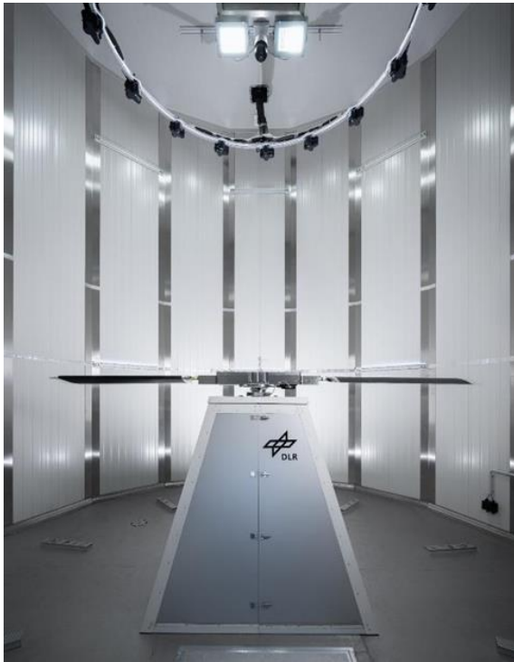
Fig. 1: Whirl tower – icing test facility © DLR
