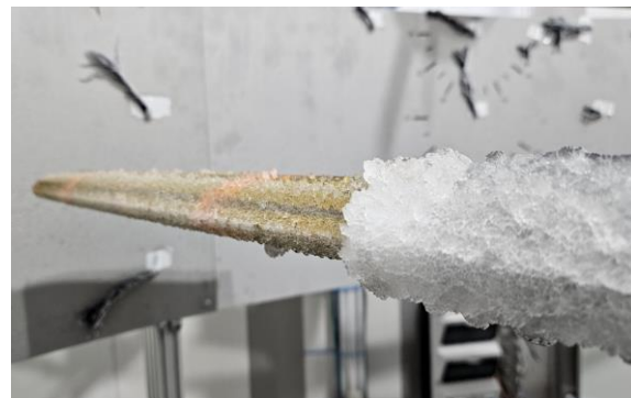
Fig. 21: Rotor blade after de-icing and icing © DLR
